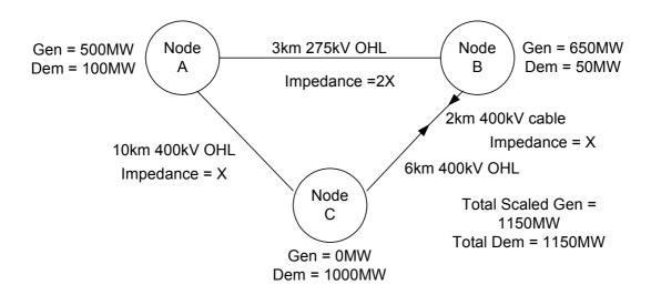
Assuming Node A is the reference node, each circuit has impedance X the 400kV cable circuit expansion factor is 10 and the 275kV overhead line circuit expansion factor is 2, the DCLF transport algorithm calculates the base case power flows as follows:
