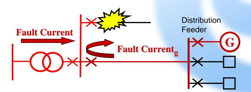
Contribution of current to a fault on network can lead to an overstressing of existing switchgear and is a major limiting factor to the connection of embedded generation
