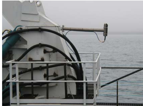
Figure 51: Current meter in position
