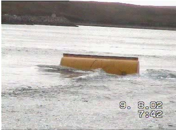
Figure 45: Effect of tidal current on mooring buoy
