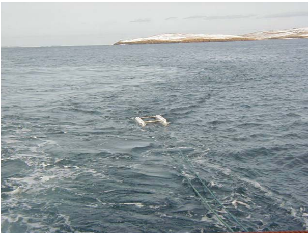
Figure 6: Sub-bottom profiling – the 'boomer'
