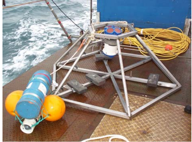
Figure 3: The ADCP and seabed frame
