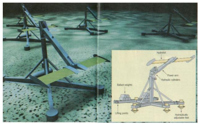
Designs incorporating two and three hydroplanes were scrapped: doubling or trebling the hydroplane area offered diminishing returns rather than delivering two or three times more lift. Again, EB weighed up cost and efficiency and calculated that a less efficient but mechanically more straightforward design would produce cheaper electricity. Stingray will be about 25% efficient, Grinsted says.
