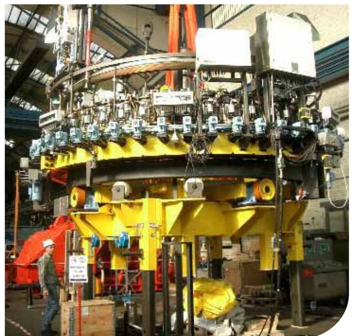
The multistud tensioning machine on its stand before the lifting test.
