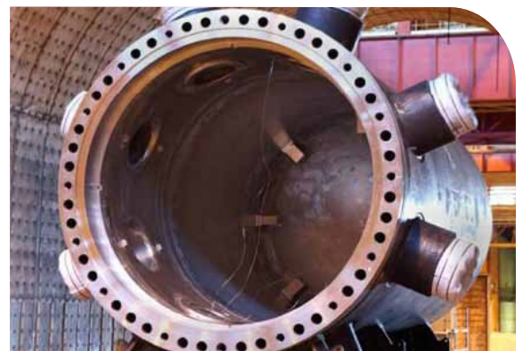
Reactor Pressure Vessel in the oven, Chalons/ St Marcel plant, France
