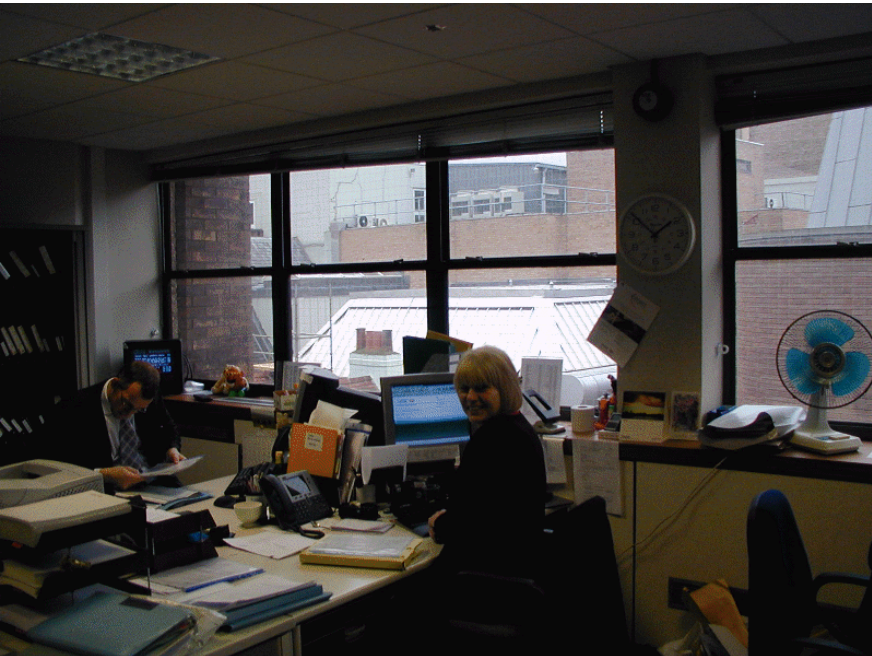
Fig. 24. The third floor office. This is smaller than the second floor and there is much more natural daylight. However, lights near the window were on during visit. A particular problem arises in this office from the glare from the roof of the building opposite seen through the window. When this photograph was taken the sun was not shining directly onto the roof.
