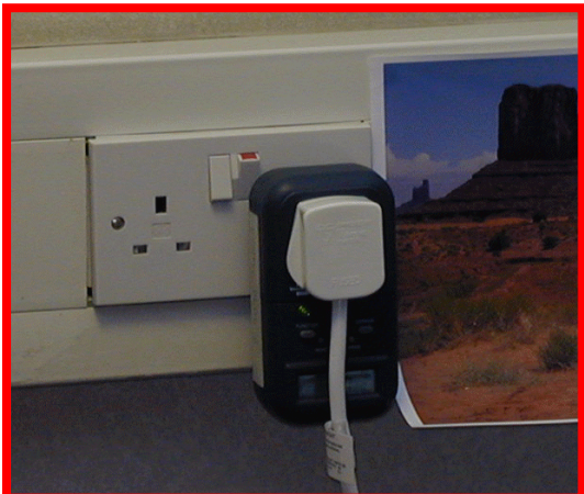
Fig. 25 A cost plug to measure electricity consumption
