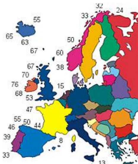
Figure 1. European Wave Resource Chart The chart shows annual average wave power in kilowatts per metre of crest width for various European sites. (Ocean Power Delivery Limited, 2005)
