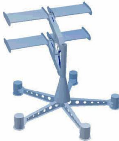
Figure 4: A computer representation of the 'Stingray' tidal stream device Source: The Engineering Business Ltd., 2003
