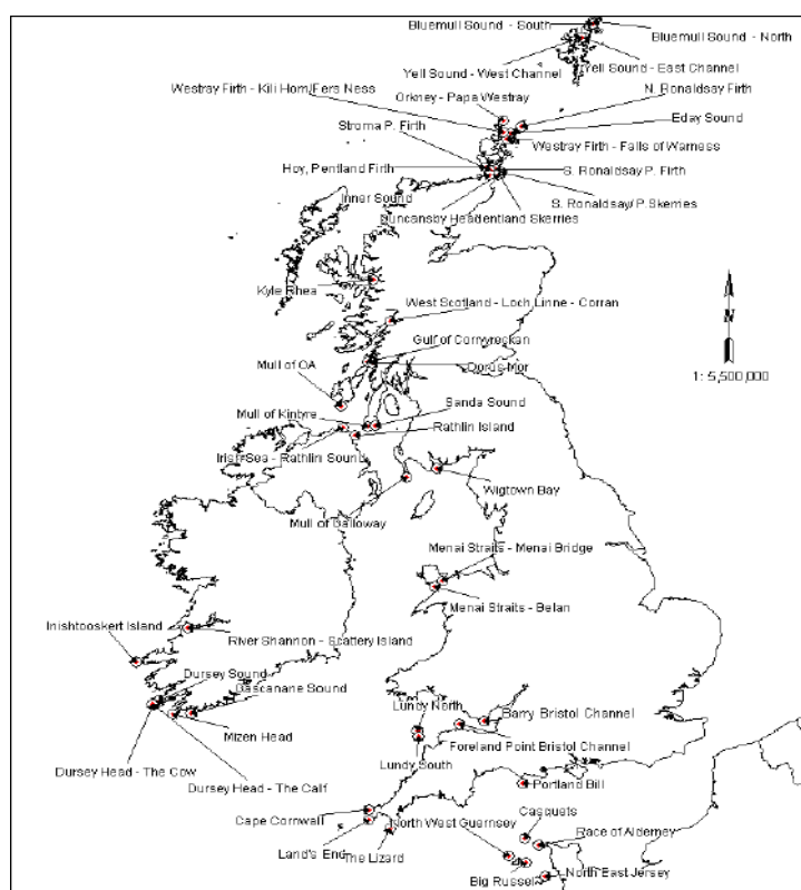
Figure 6: The location of suitable tidal stream energy extraction sites Source: The Carbon Trust 2004
