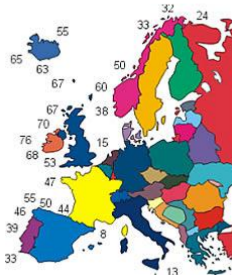
Figure 1: European Wave Resource Chart showing the annual average wave power in kW/m of crest width for various European sites. (Ocean Power Delivery Limited)
