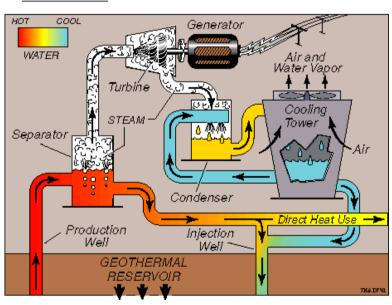
the range 150-300°C (300-700°F). For these systems, flash-steam power plants are required. Again, the geothermal fluids are brought to the surface through production wells as much as 4 km deep.
