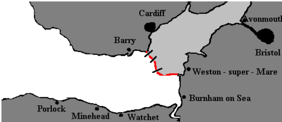
Fig. 17.4 A proposed single basin scheme
