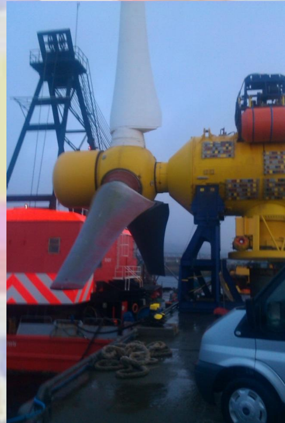
1MW Tidal Stream Alstom device on Hatston Quay, Orkney in April 2013.
