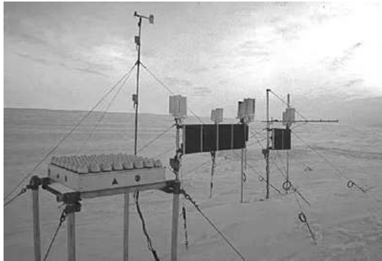
Figure 2.7: Photograph of the Doppler sodar wind profiler. The actual profiler is visible in the foreground (on the left), in the background the solar panels, wind generators, radio antenna and AWS mast are visible. Photo courtesy Ian Renfrew.
