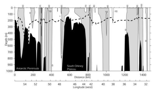
**Figure 2d.** As in Figure 2a but for geostrophic velocity (cm s<sup>-1</sup>) referenced to the lowered acoustic Doppler current profiler profiles. Contour interval is 10 cm s<sup>-1</sup>, and northward (positive) values are shaded gray.
