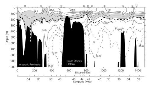
**Figure 2b.** As in Figure 2a but for salinity. Contour interval is 0.1, and values between 34.3 and 34.5 are shaded gray. The thin dashed contours are 34.65 and 34.67 for added detail in the Warm Deep Water.
