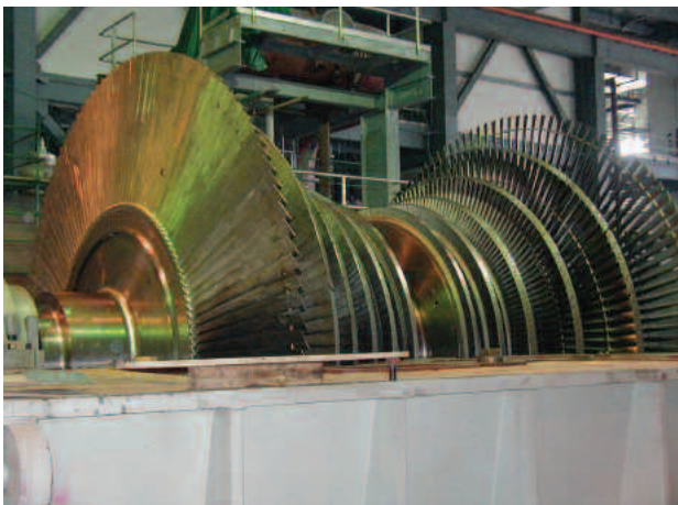
Figure 2-22 Qinshan Low-Pressure Turbine Rotor
